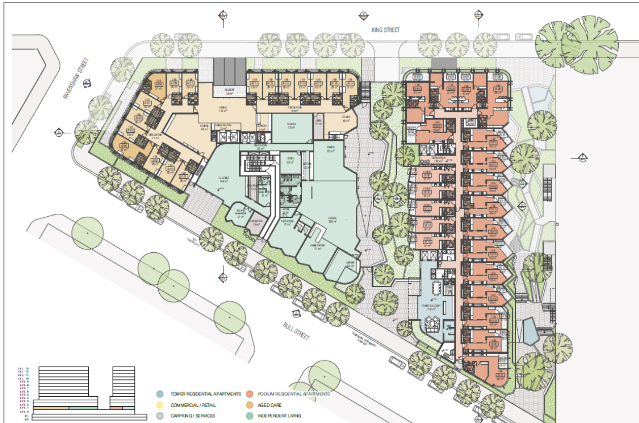
Figure 3: The podium and tower levels are appropriately separated in compliance with ADG requirements to reduce the buildings' appearance of bulk and scale at street level, maintain appropriate visual privacy and solar access, and to facilitate extensive landscaping and pedestrian connectivity. The laneway between the adjacent Wests City building on the east provides an attractive and high-quality contribution to the public domain.
